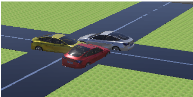
Figure 8: Three Hybrid Change & Keep and Change-or-Learn-Fast agents enacting behavior that leads to a ‘Crash’ outcome. In early episodes, car agents are still exploring and will often fail to appropriately reduce speed, which is acting ‘selfish’, leading to crashing into each other and a low collective payoff.
